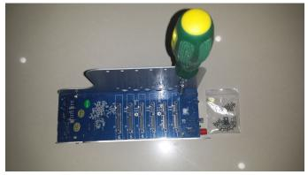
5. Photo shows both side plates installed ... time to tighten all 8 screws.
